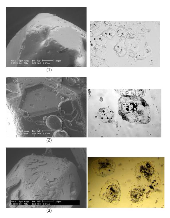
**Figure 4** ESEM and optical images of the medium-sized (class 1) material. The most sensitive (1) is shown at the top and the least sensitive (3) is at the bottom. The field of view of the optical images is 0.6mm wide.
