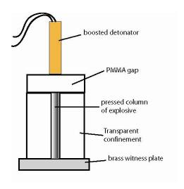
**Figure 1**. Diagram of the small-scale gap test. The charge was 5mm in diameter and 25mm long, contained within 25mm diameter PMMA.
