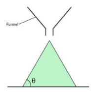
**Figure 5**: Schematic representation of the angle of repose. The material is poured though a funnel to form a conical pile and the angle between the horizontal and the side of the pile is measured.
