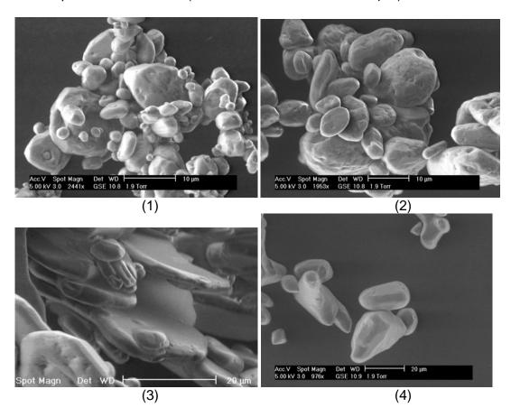
**Figure 3** ESEM images of the four RDX products of the smallest size class. (1) is the most sensitive and (4) is the least sensitive. (1) has many micronsized dimples, which may be the cause of its high sensitivity.
