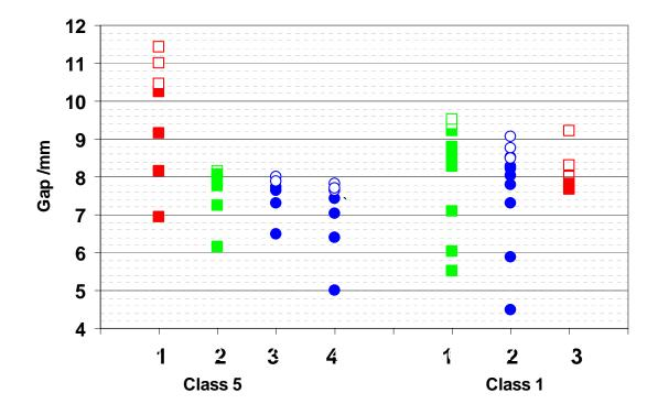
**Figure 2**: Gap test results for class 5 (10-30 $\mu$ m) and r class 1 (100-300 $\mu$ m) batches. Open symbols represent "no go" events and filled symbols represent "go" events.
